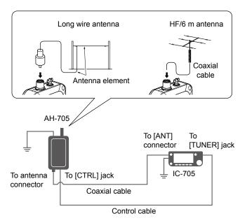
⚠ **DANGER HIGH VOLTAGE! NEVER** touch the antenna element while tuning or transmitting. Always install the antenna element in a secure place.
