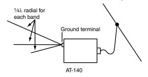
$1/4\lambda$  (quarter wavelength) radial for each band is suitable for a counterpoise. Install the counterpoise directly below the AT-140's ground terminal. Insulate the ends of each radial from other metal objects. Layout the radial horizontally and as straight as possible.
